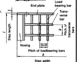
Designation of a tread with a type SP grating in compliance with this standard, where h is equal to 40 mm, a is equal to 38,1 mm, l is equal to 800 mm and b is equal to 240 mm:
