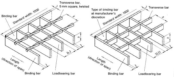
Designation of a type SP grating complying with this standard, where h is equal to 40 mm, a is equal to 38,1 mm, with a length in the direction of span (T) of 800 mm and a width of 1000 mm:
